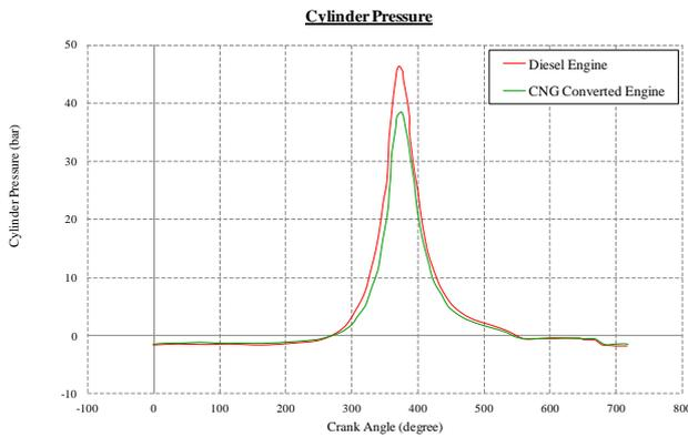
**Figure 15:** The values of Cylinder Pressure ( $P$ , bar) is determined via testing result between diesel engine and CNG converted engine vs Crank Angle (degree),  $P_{max}$  (CNG converted engine) is approximately 39bar at TDC (720 degree)
