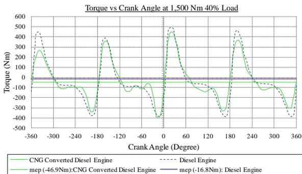
**Figure 17:** The Comparison Engine Torque Values between CNG Converted Engine and Diesel Engine at 1,500RPM with Additional 40% Total Truck Load vs Crank Angle
