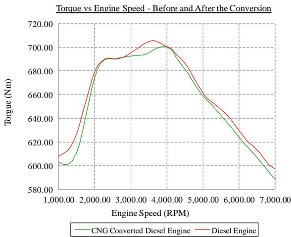
**Figure 16:** The Performance Curve (Torque vs Speed), Before and After the Conversion (Source: the Result from this Project)
