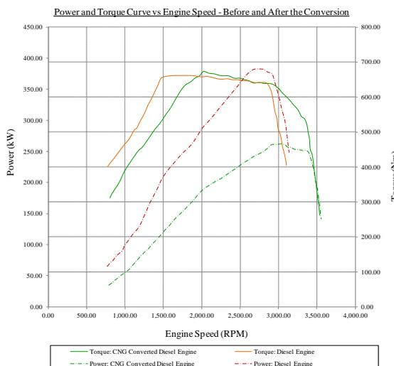
**Figure 21:** The simulation results of the power and torque versus the engine speed before and after the conversion
