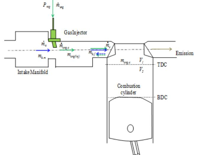
**Figure 10:** The Schematic Diagram for the CCDE with Backlash
