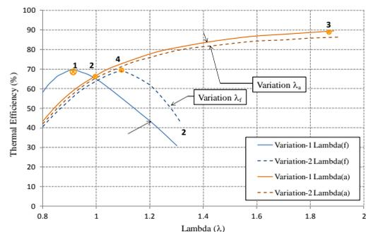
**Figure 4:** The Affect of the Thermal Efficiency ( $\eta_e$  %) due to the Variation Values of  $\lambda_f$  and  $\lambda_a$  1. Maximum Power Input, 2. Stoichiometric Ration, 3. Diesel and Lean – Burn Engines, and 4. Moderately Lean Operation (after, Kiencke & Nielsen, 2005)
