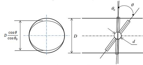
**Fig-3:** The Throttle Geometry
