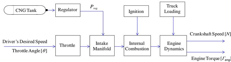
**Figure 19:** The Opened-loop Schematic Processing Flow for the CCDE System
