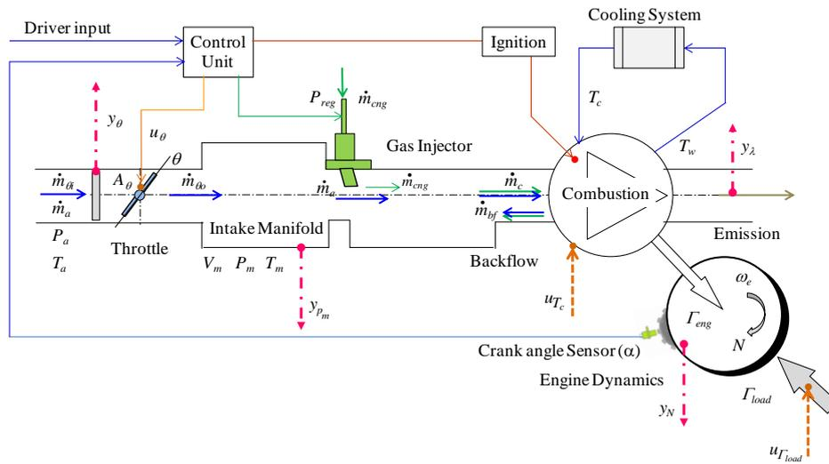
**Figure 18:** The overall Schematic Flow Diagram for the CCDE
