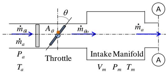
**Figure 7:** The Schematic Flow Diagram at Throttle & Intake Manifold
