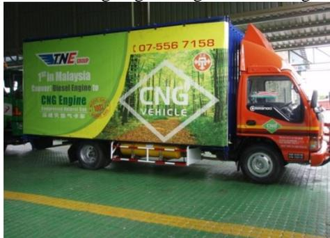
**Figure 1:** The First Working Prototype which is powered by a CNG Conversion Diesel Engine – Engine Type: HICOM PERKASA MTB150 Engine, Model 4HF1, 4,300cc.
