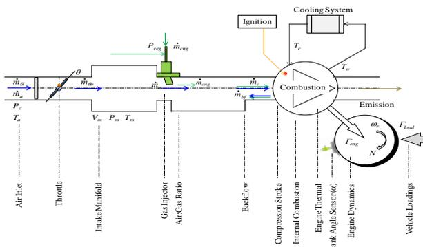
**Figure 2:** The Schematic Diagram for the whole CCDE system and sub-systems
