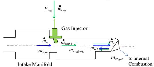
**Figure 6:** Gas Injector at the Intake Manifold
