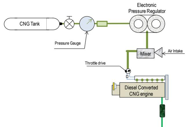
**Figure 8:** The Combination System of the CCDE
