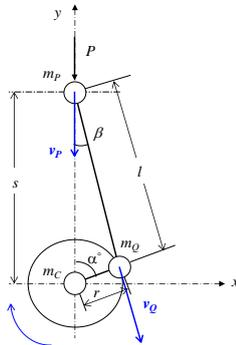
**Figure 13:** The Assumption of Total Mass for the Mechanism of the Dynamics System Model
