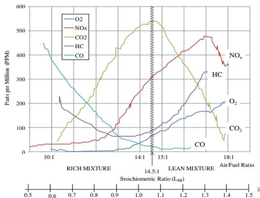
**Fig-5:** The Emission Values in Parts per Million (PPM) based on the Air/Fuel Ratio and the Required Stoichiometric Ratio ( $L_{SR}$ ) (Heywood J. B., 1988).
