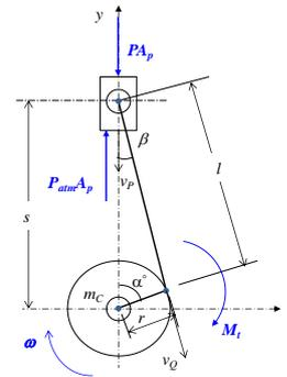
**Figure 14:** The Exerted Power and Moment of Force Modelling on the Dynamics Mechanism System
