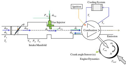
**Figure 9:** The Schematic Flow Diagram from the Manifold Outlet to the Engine Dynamics
