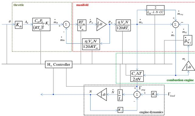
**Figure 20:** The Closed-Loop Control Model for the CCDE
