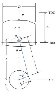
**Figure 11:** The Geometrical Diagram for the Engine Variables such as Piston, connecting Rod ( $l$ ), Crank Radius ( $r$ ), Crank Angle ( $\alpha$ ), Bore ( $D$ ), Stroke ( $s_{st}$ ) and Distance between the Crank Axis and the Piston Pin ( $s$ )
