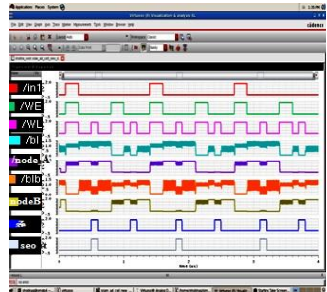
Figure 1.5: Waveforms of Asymmetrical 1 bit Adiabatic SRAM cell
