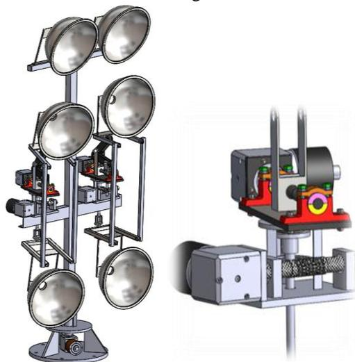
The simplified CAD Model of Mechanism consisting of a Leadscrew, Gearbox and Plummer block is as shown in the
