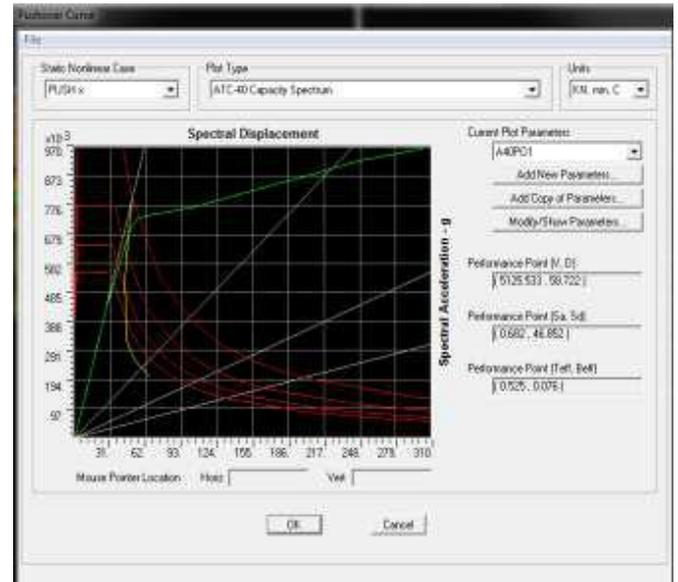
**Figure 5:** Performance point due to PUSH X
