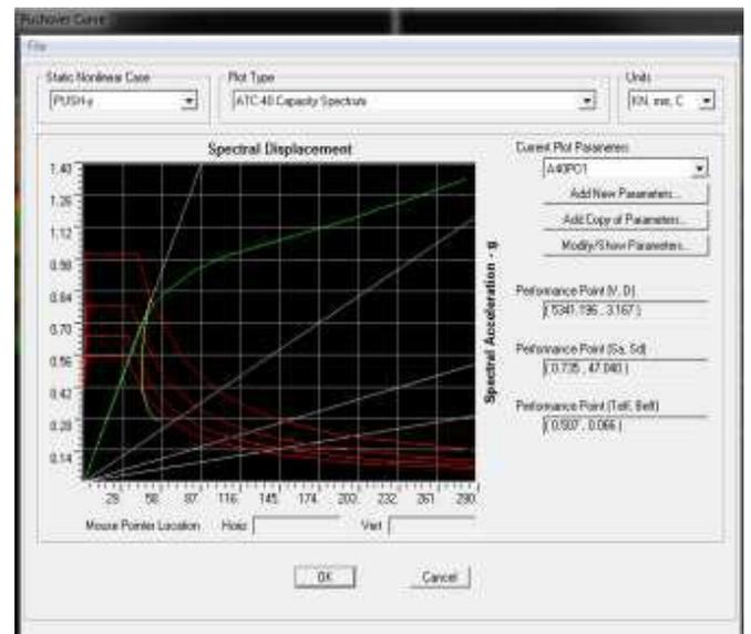
**Figure 6:** Performance point due to PUSH Y
