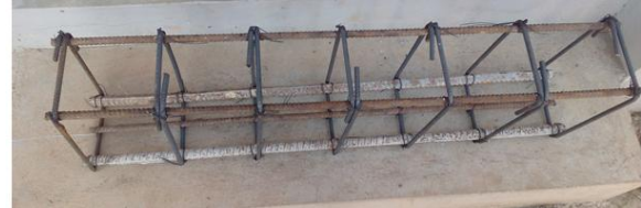
Figure 1: Reinforcement Cage for Beam Specimens
