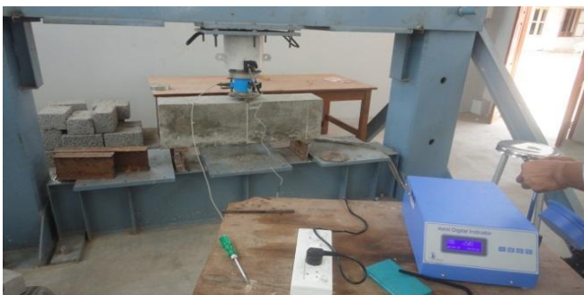
Figure 7: Experimental Setup of Beam Specimens
