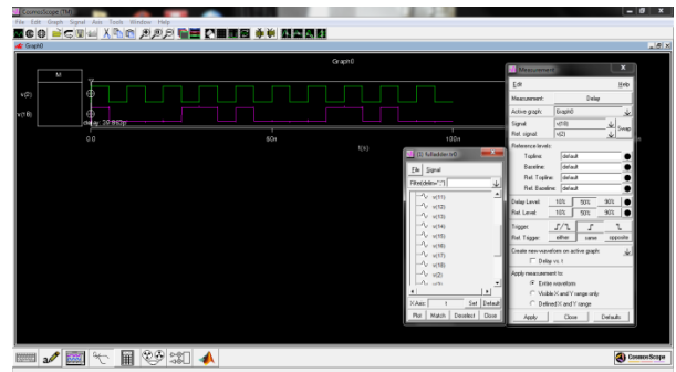
Figure 9: Delay calculation of Proposed Full adder design in 90nm technology.
