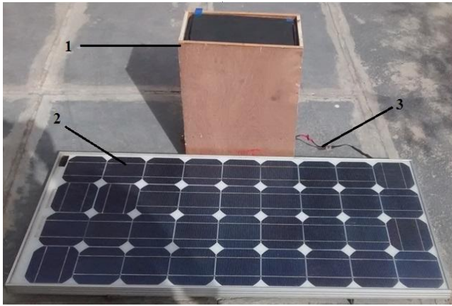
Figure 4: Fabricated Thermo Electric Refrigerator system powered by solar energy
