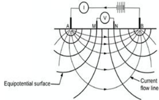
**Figure 2:** Illustration of surface resistivity method showing simplified current flow lines and equipotential surfaces arising from a set of current electrodes (A/B and M/N respectively)
