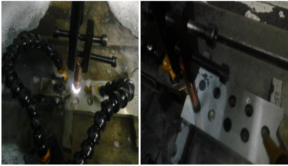
Figure: Spark produced between tool and work piece during machining
