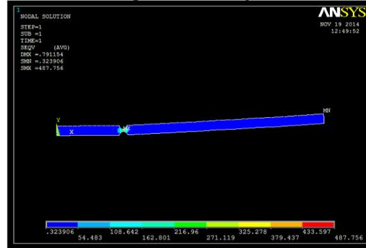
**Figure 6:** Deflection of lumped beam.
