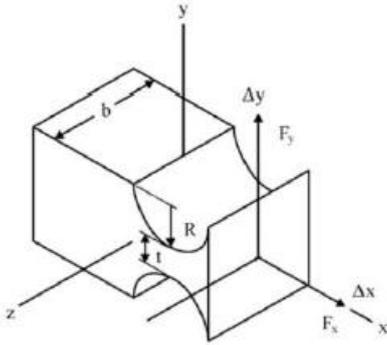
**Figure 1:** Flexure hinge [7]
