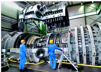
Stationary gas turbine
