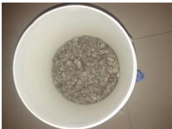
Figure 1: 5-4 cm size of gravel used in formation of vermifilter bed
