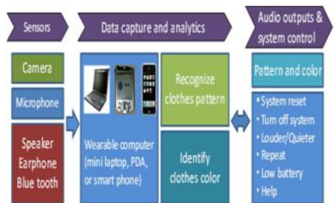
Figure 1: Overview and architecture design of camera based system
