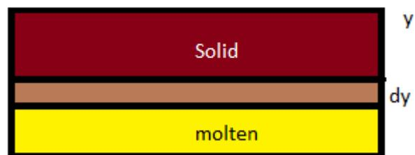
For an additional layer of thickness  $dy$  of crust to form in some small time  $dt$ , some  $dQ$  amount of heat has to leave this layer, and be conducted through the crust formed into space. From the principles of Calorimetry we have:
