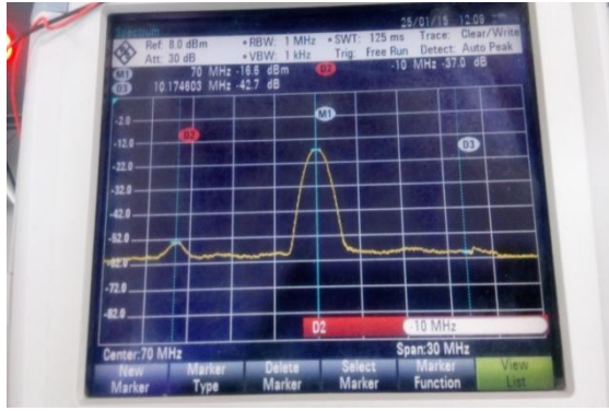
Figure 8: Input data signal without spreading at a rate of 10 Mhz.
