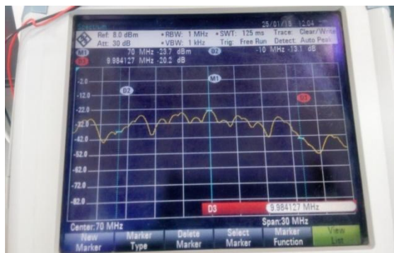
Figure 9: Input data signal without spreading at a rate of 10 Mhz
