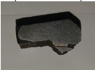
Figure 2.3: etched sample of 1x1" sample of drum brake
