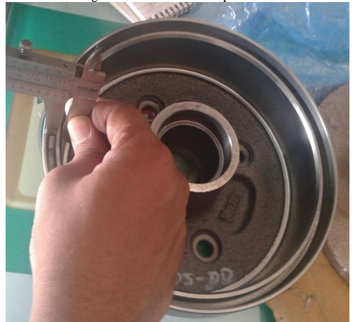
Figure 2.1: New Drum brake for Ra value
