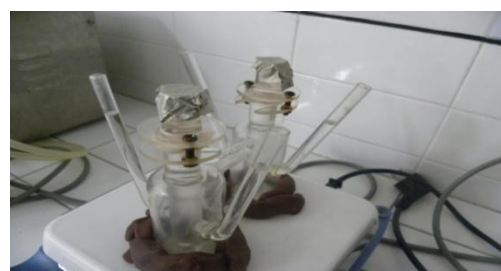
Figure 1: permeation skin test using Franz like diffusion cell
