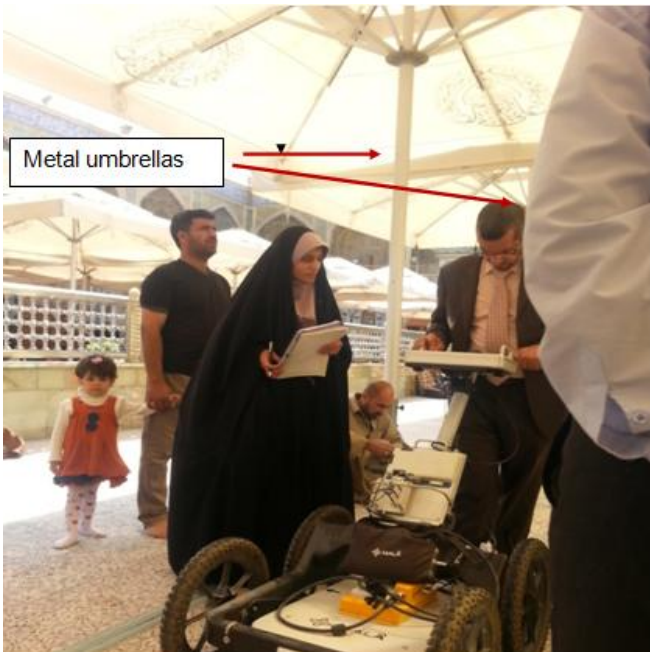
Figure 4: Shows umbrellas that cause the emergence anomalies in the profile (344)
