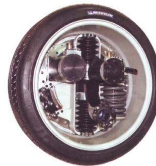
Figure 11: Michelin designed active wheel with an active suspension system.
