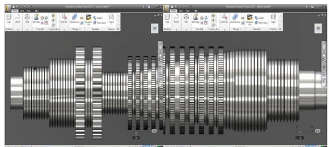
Figure 2.4: 3-D Model of a LP 80MW STEAM TURBINE ROTOR
