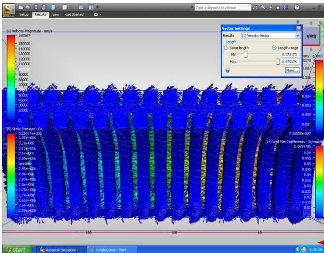
**Figure 3.1:** Results of CFD Analysis for Cr-Mo Steel Labyrinth seal.
