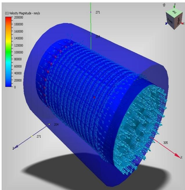
**Figure.3.2:** Results of CFD Analysis for Si-C Labyrinth seal
