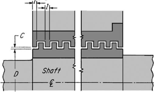
Fig.2.1. Labyrinth seal with a turbine shaft
