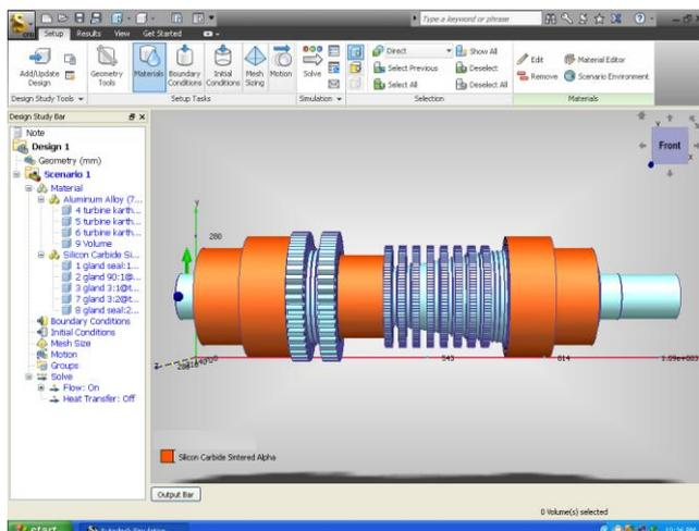
**Figure 2.6:** 3-D Model of a LP 80MW STEAM TURBINE ROTOR with Labyrinth seal imported into CFD Software
