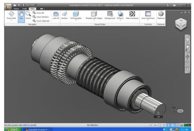
Figure 2.5: 3-D Model of a LP 80MW STEAM TURBINE ROTOR with Labyrinth seal
