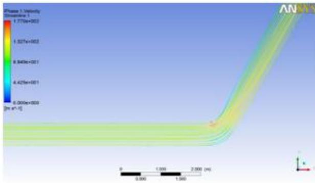
Figure 2: Streamlines of 120° Bend
