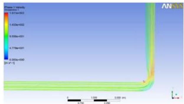
**Figure 1:** Streamlines of 90<sup>0</sup> Bend
