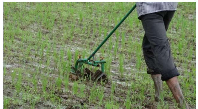
Figure 3: Photographic view of cono weeder working in the field
