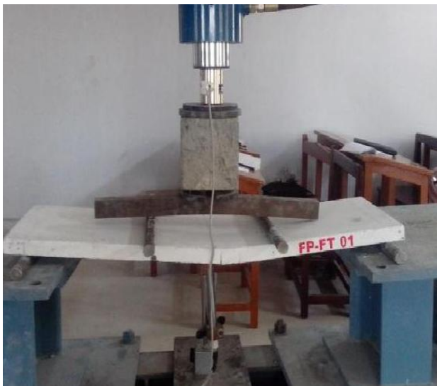
Figure 7: Testing of slab FP-FT 01
