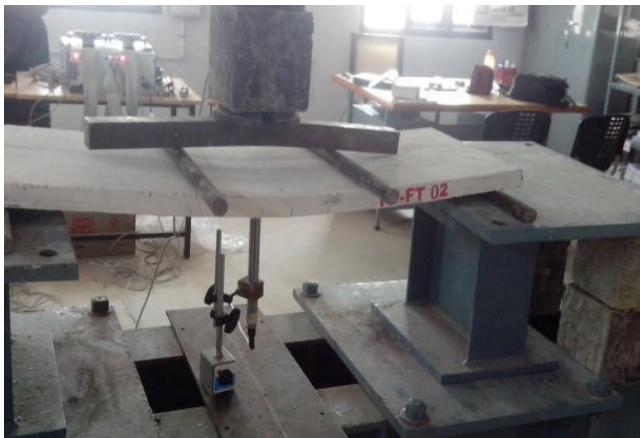
Figure 8: Testing of slab FP-FT 02
