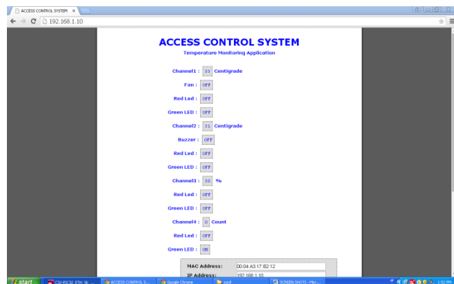
Figure 6: WEB Page for monitoring from remote location
