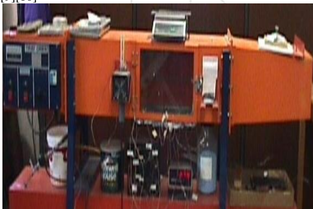
Figure 1: Tray Dryer used for the unit operation on the bacterial cellulose
