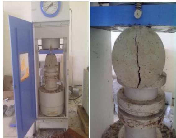
Figure 3: Testing the Cylinder Specimen
