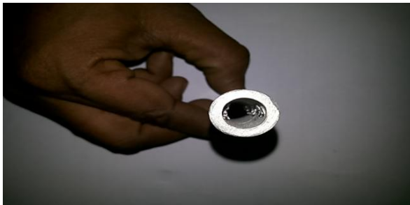
Figure 6: Perforated Pin Fin used for the purpose
