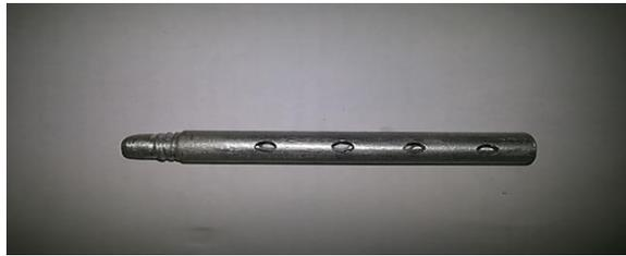
Figure 6: Perforated Pin Fin used for the purpose
