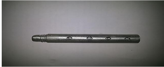
Figure 6: Perforated Pin Fin used for the purpose
