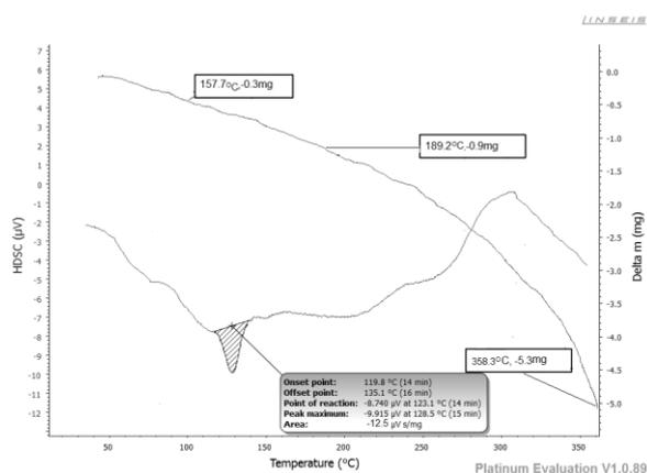
**Figure 6: TG/HDSC Thermogram of L2-Ni**
