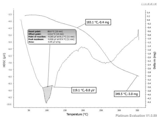
Figure 8: TG/HDSC Thermogram of L3
