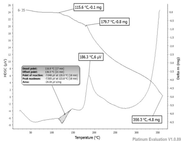
Figure 7: TG/HDSC Thermogram of L2-Ag
