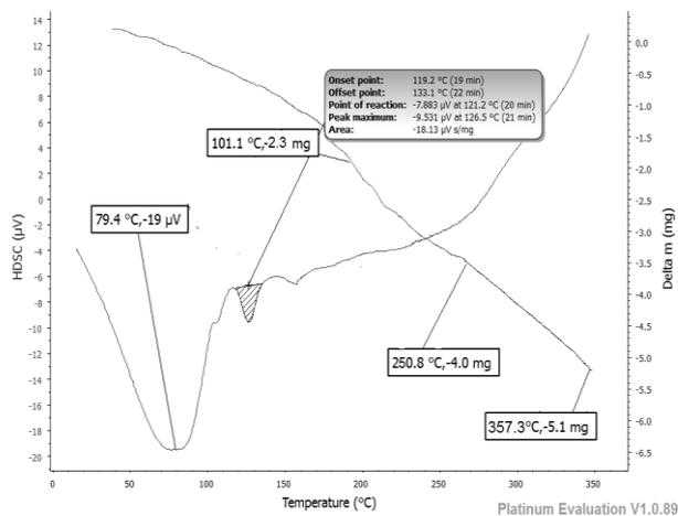
Figure 9: TG/HDSC Thermogram of L3-Pd
