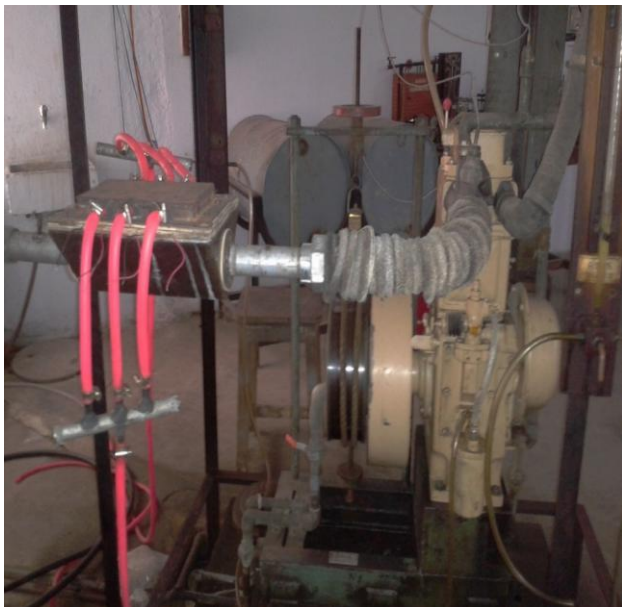
Figure 4: Assembly of TEG to a Compression Ignition engine.
