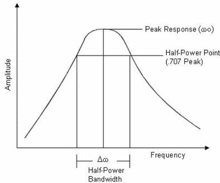
**Figure 1:** Frequency Response Function
