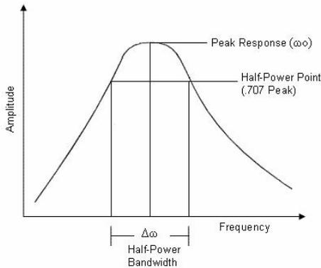
**Figure 1:** Frequency Response Function
