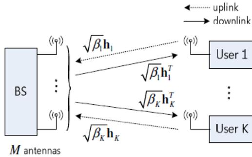
Fig. 1. TDD multiuser MIMO system model.
