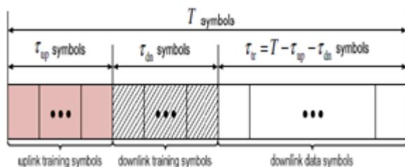
Figure 2: Frame structure of TDD system for downlink
