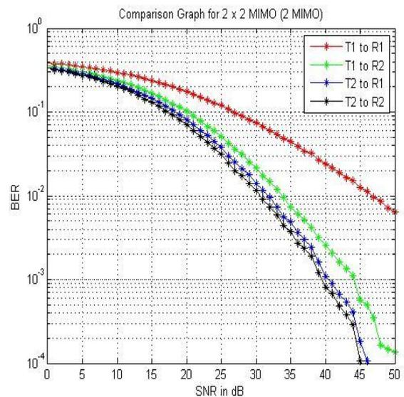
**Figure 10:** Comparison Graph for 2x2 MIMO
