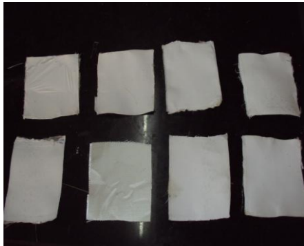
Figure 6: Electrospun Nylon 66 fibers on glass fiber 7781
