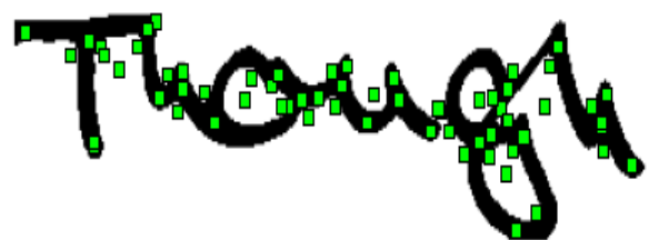
Figure 3: The key points detected in a word region by SIFT.
