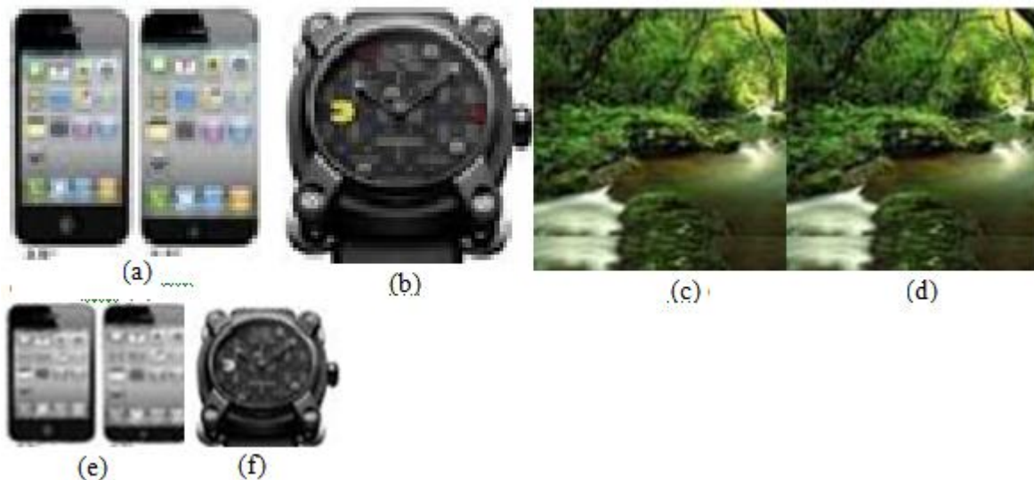
Figure 4: Chang's secret sharing algorithm results: (a) cover image 1, (b) cover image 2, (c) secret image, (d) reconstructed image, (e) camouflage 1, (f) camouflage 2
