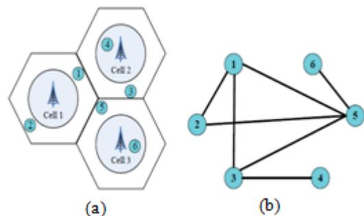
**Figure 2:** An example of the graph-based framework. (a) 3cell scenario. (b) Interference graph construction
