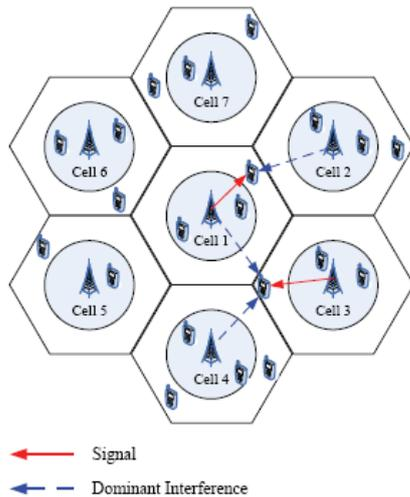
**Figure 1:** An example of an LTE network with inter-cell interference
