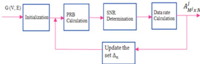
**Figure 3:** Block diagram of PRB allocation
