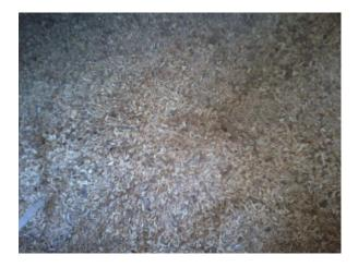
Saw dust concrete consist of roughly equal parts by volume of Portland cement, sand and pine saw dust, with water to give a slump of 25 to 50 mm. it bonds well to ordinary concrete and is a good insulator.
