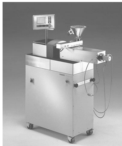
Figure 1: Torque rheometer with a twin-rotary mixer
