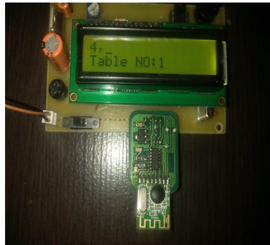
Figure 5.6: ordered item and table no. at kitchen unit
