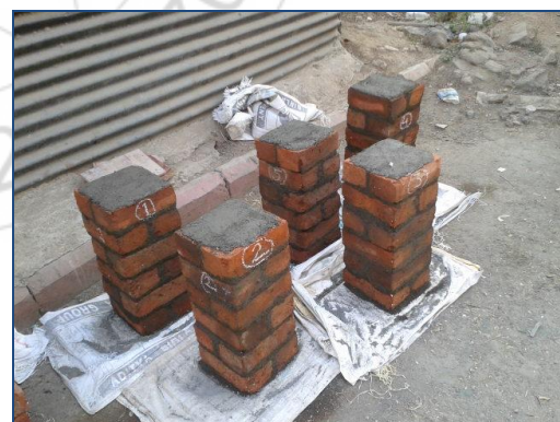
Figure 3: Brick Masonry Prisms
