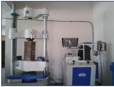
Figure 4: Testing of Brick Masonry Prism
