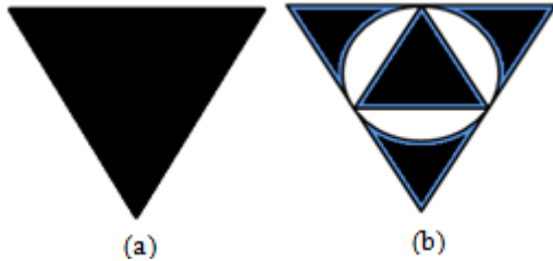
Figure 3: Proposed compound fractal antenna (a) Initiator (b) Generator.
