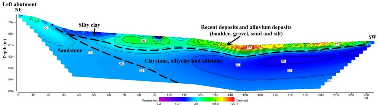
Figure 9: Inverse resistivity model along profile 1 which is parallel to the proposed dam axis
