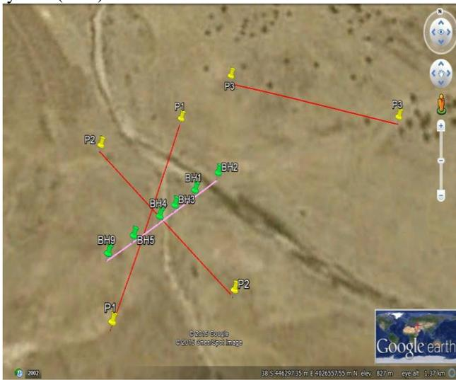
**Figure 8:** Image shows the field survey layout and location of boreholes at Shaqlawa proposed dam site.
