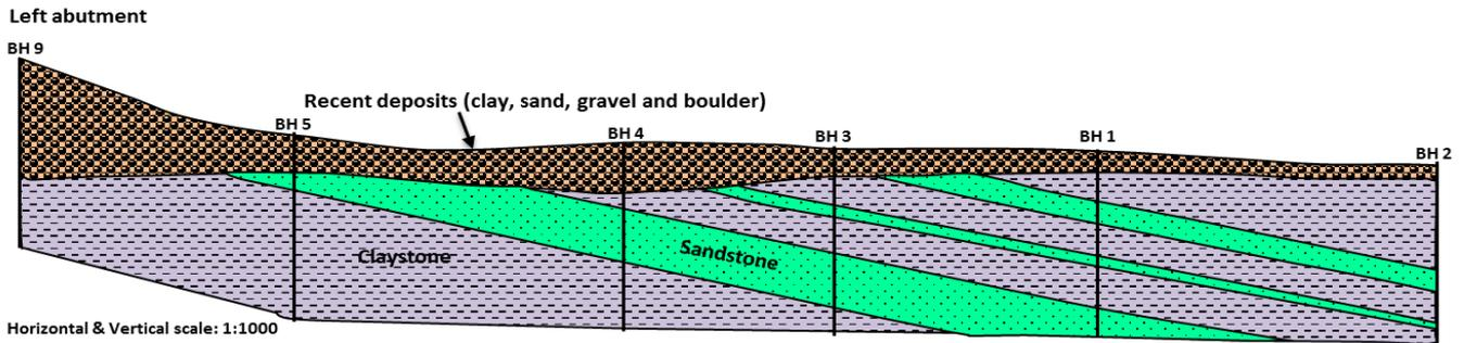
Figure 10: Boreholes lithological correlation along the dam axis [27].
