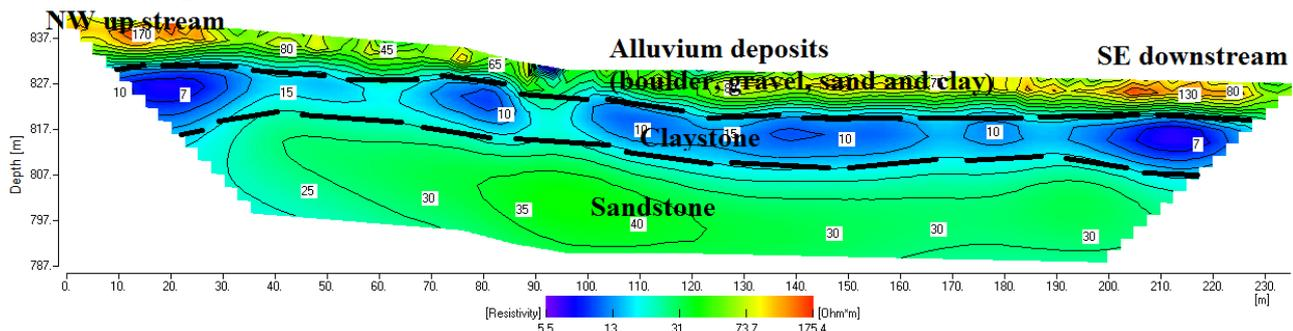
Figure 11: Inverse resistivity model along profile 2 which is perpendicular to the proposed dam axis.
