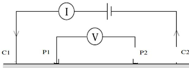
**Figure 6:** General four electrode configuration for resistivity measurement [16].
