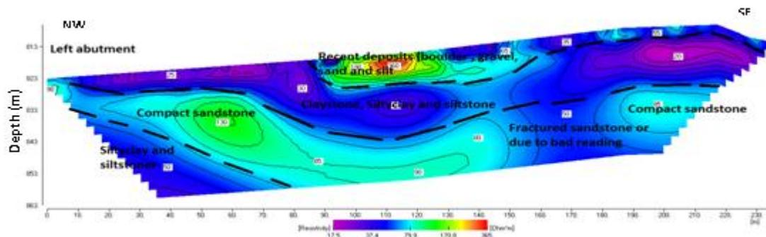
Figure 12: Inverse resistivity model along profile 3 which is on the right abutment of the proposed dam.
