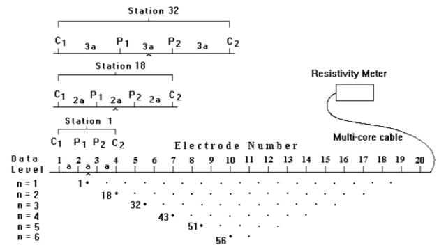
**Figure 7:** A typical field arrangement for 2D ERT Surveys (Wenner array) [19].
