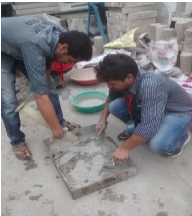
Figure 1: Mixing of concrete
