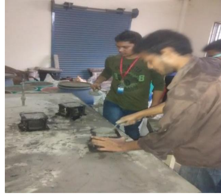
Figure 2: Demoulding of concrete
