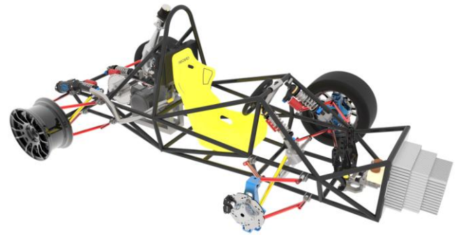
Figure 6: Full Car Assembly Model
