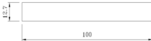
Figure 5: Bending test sample Dimensions
