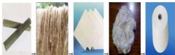
From left to right: (1) raw bamboo is gathered, (2) bamboo is crushed and processed into thick pulp (raw chemical bamboo fibre) (Pure Fiber 2008), (3) bamboo is further processed into fine pulp sheets, (4) bamboo pulp is manufactured into fibre through wet spinning process, (5) bamboo fibres are spun into yarn
