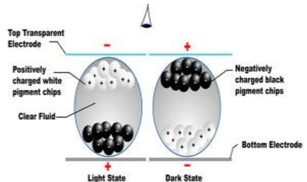
**Figure 2:** It show that when a voltage is applied, the particles will migrate eclectically to the plate bearing the opposite charge from that on the particles
