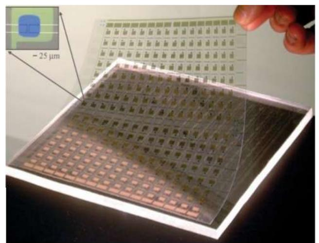
**Figure 3:** Basic scheme of an Electrophoretic Display using color filters and Rubber Stamped Plastic Circuitry for Electronic Paper
