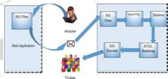
Figure 1: Information flow in an mXSS attack.
