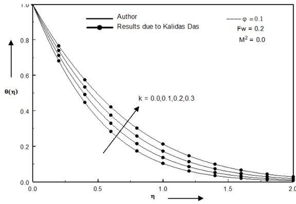
**Figure 3:** A comparative study of Temperature distribution for various values of  $k$  (For Copper-water nanofluid)
