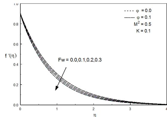
**Figure 13:** Velocity for various values of injection parameter (For Alumina-water nanofluid)
