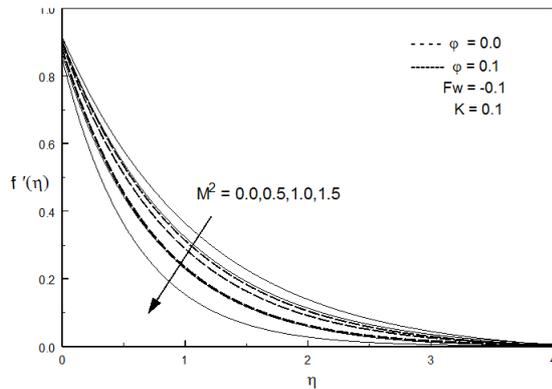
**Figure 4:** Velocity profiles for various values of  $M^2$  (For Copper-water nanofluid)
