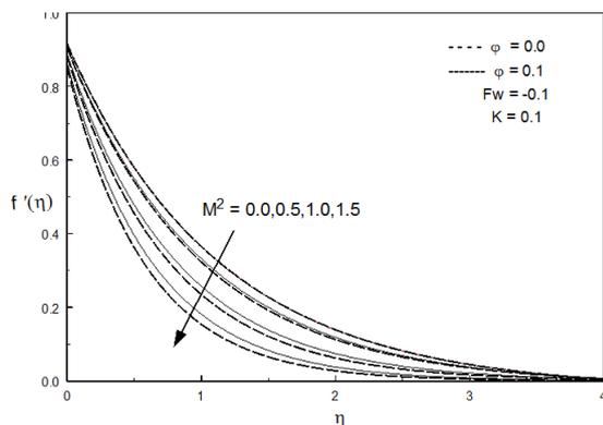
**Figure 5:** Dimensionless streamwise velocity profiles for various values of  $M^2$  (For Alumina-water nanofluid)
