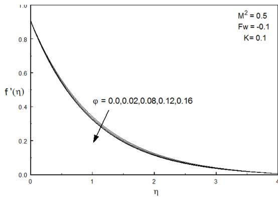
**Figure 17:** Effect of volume fraction over non-dimensional streamwise velocity (For Alumina-water nanofluid)
