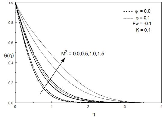
**Figure 6:** Temperature distribution for various values of  $M^2$  (For Copper-water nanofluid)
