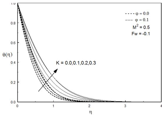
**Figure 10:** Temperature distribution for various values of  $k$  (For Copper-water nanofluid)
