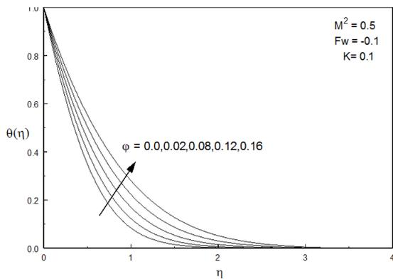
**Figure 18:** Temperature distribution for various values of  $\phi$  (For Copper-water nanofluid)
