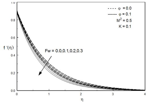
**Figure 12:** Velocity for various values of injection parameter (For Copper-water nanofluid)
