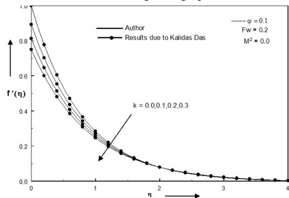
**Figure 2:** A comparative study of dimensionless streamwise velocity for various values of k (For Copper-water nanofluid)
