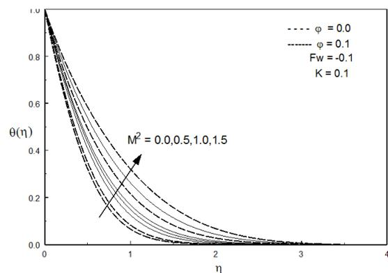
**Figure 7:** Temperature distribution for various values of  $M^2$  (For Alumina-water nanofluid)
