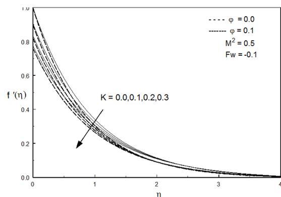
**Figure 8:** Velocity profiles for various values of  $k$  (For Copper-water nanofluid)
