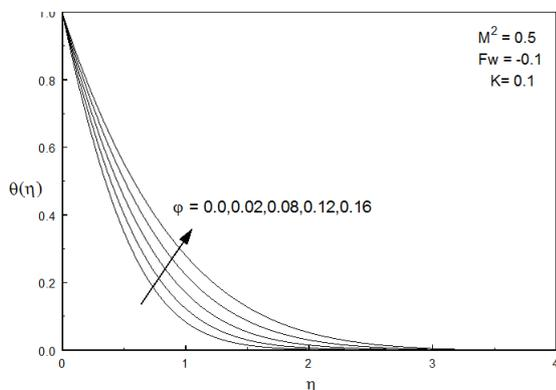
**Figure 19:** Temperature distribution for various values of  $\phi$  (For Alumina-water nanofluid)
