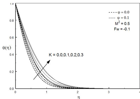
**Figure 11:** Temperature distribution for various values of  $k$  (For Alumina-water nanofluid)
