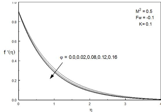
**Figure 16:** Effect of volume fraction over Velocity (For Copper-water nanofluid)
