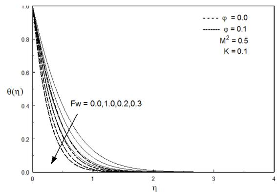
**Figure 14:** Temperature distribution for various values of injection parameter (For Copper-water nanofluid)
