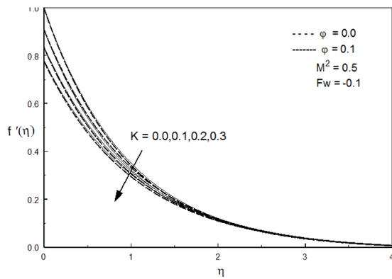
**Figure 9:** Dimensionless streamwise velocity for various values of  $k$  (For Alumina-water nanofluid)
