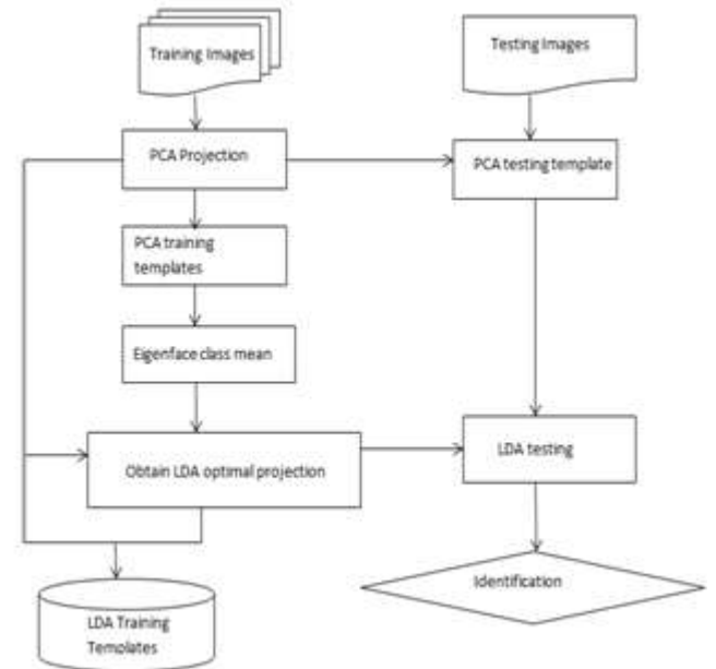
Figure 3: Simple flowchart of PCA algorithm
