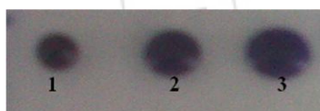
Figure 1: Drop collapse assay indicating biosurfactant production (1- water, 2-test bacterial culture supernatant, 3- SDS solution)
